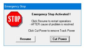
Clicking on **Resume** cancels the Emergency Stop of all Items, although each Item will remain stationary on the track until a new speed command is sent from the Controller (NCE Cab or Operate 'soft controller') to which that Item is allocated.
