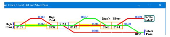
Although, in general, a route cannot include any occupied blocks, you **can** select an occupied block as Route Start, **provided** that this starting block does **not** include a turnout in its exit path.
